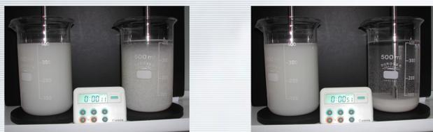
Sedimentation of 5 g/dm<sup>3</sup> kaolin suspension without and with 10 ppm starch based flocculant
